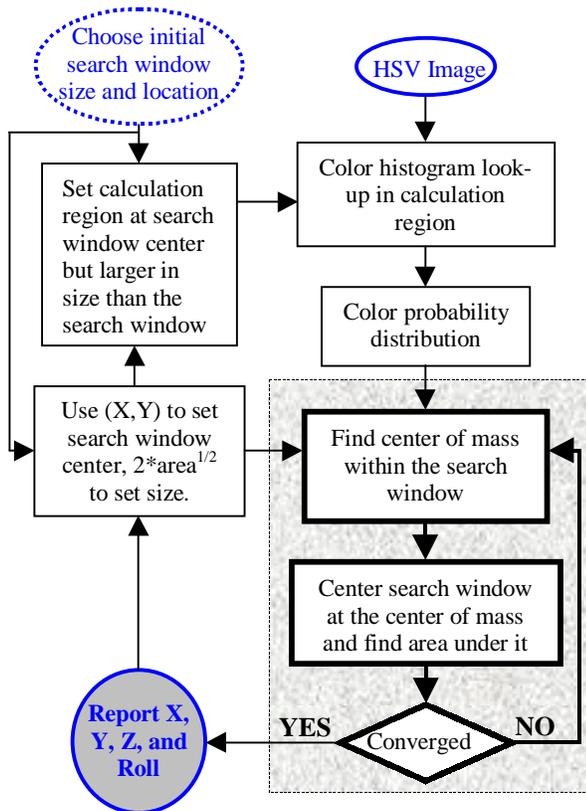
Figure 1: Block diagram of color object tracking
