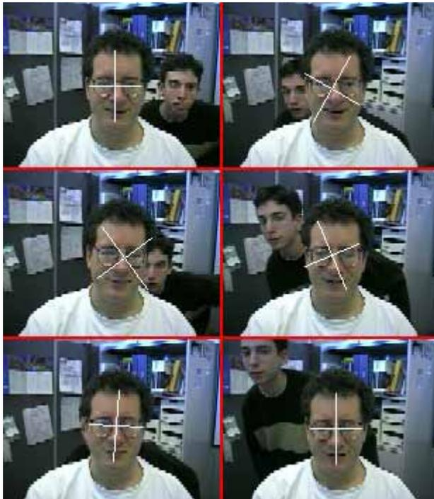
**Figure 17:** Tracking a face with background distractor faces (sequence: down left then right columns)
